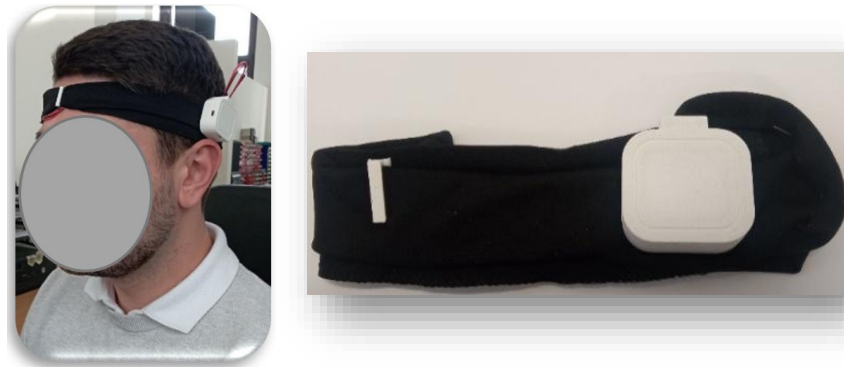
Figure 3: Realized a wearable device for measuring body temperature
